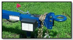
Optional Equipment: Heavy Duty Tongue with Adjustable Height Pintle Hitch, Safety Tow Chains, Lights, Electric Brakes and Tongue Jack.
