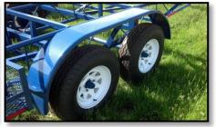
Optional Equipment: 3500 Lb. Tandem Axles, 15" Highway Speed Radial Tires on 5 Bolt White Spoke Wheels and Fenders.
