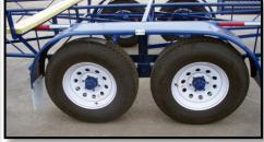
Optional Equipment: 6000 Lb. Tandem Axles, 16" Highway Speed Radial Tires on 6 Bolt White Spoke Wheels, Fenders with Splash Guards, D.O.T. Conspicuity Tape and Treated Wood on Cross Members.
