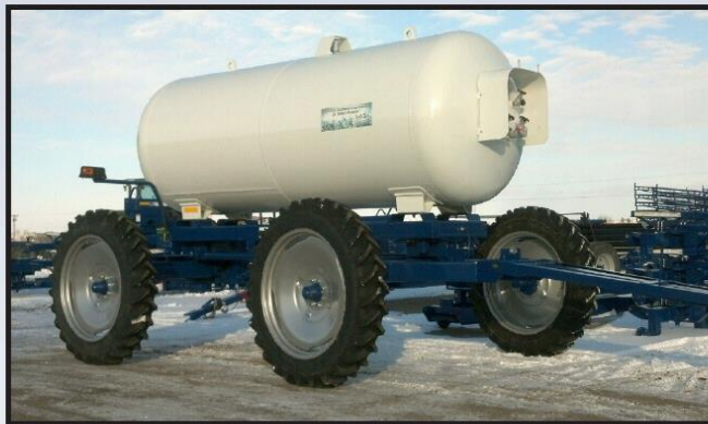
DS2110 with Optional 2000 Gallon NH3 Tank and 320/85R38 Tires
