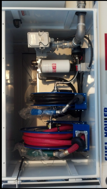
12V, 20 - 25 GPM Diesel Pumping System with 50 Gallon D.E.F. Tank
